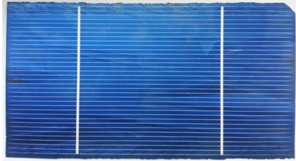
Figure 18. Ribbon growth (EFG) Si solar cell.
