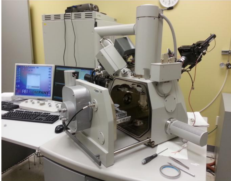
Figure 21. FEI Quanta 200 3D dual system.
